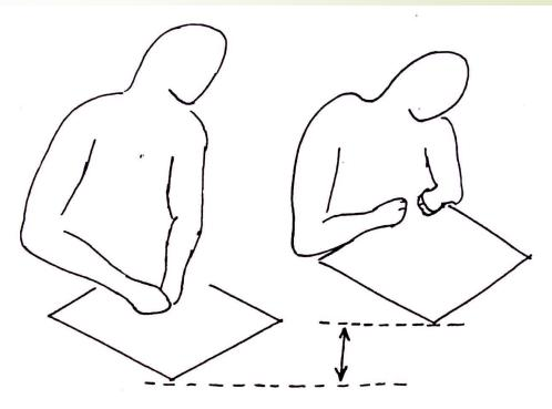
Figure 7. Higher work-bench for finer work.
